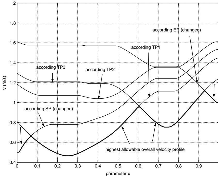
Fig. 9. The corrected velocity profile concerning initial and terminal velocity.
