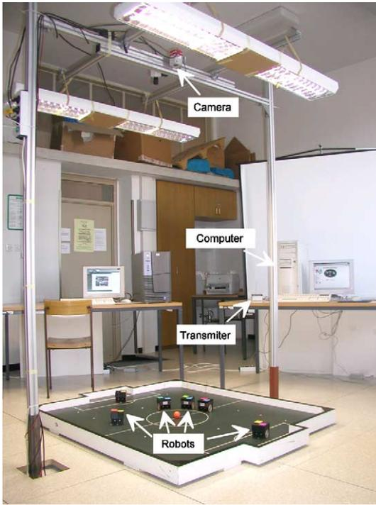
Fig. 1. The robot soccer system.
